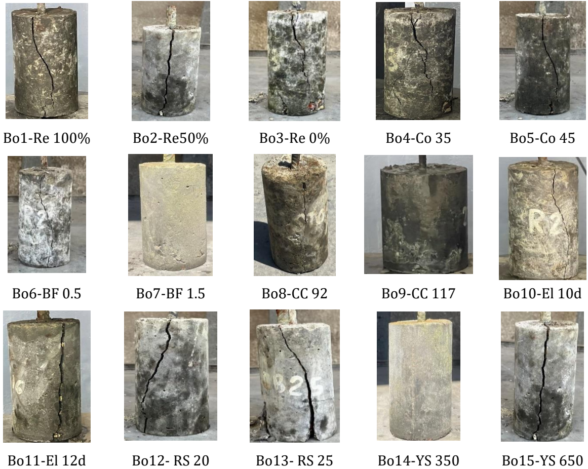
Fig. 5. Failure modes of all tested specimens
