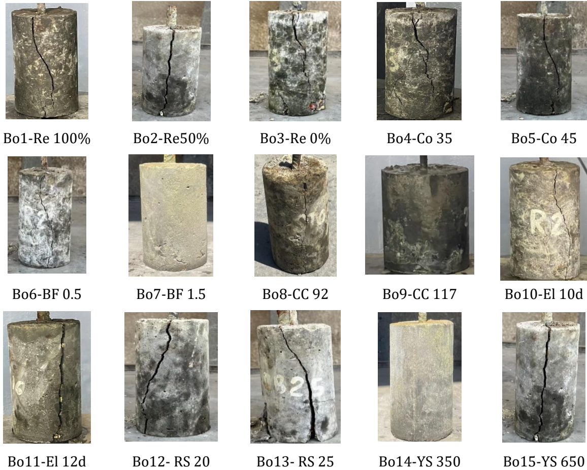
Fig. 5. Failure modes of all tested specimens
