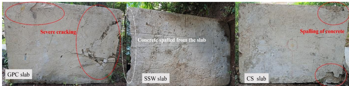
Fig. 14. Failure pattern of the Slab elements
