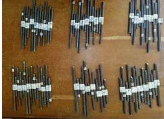
Fig. 4. Rebar samples after fracture
