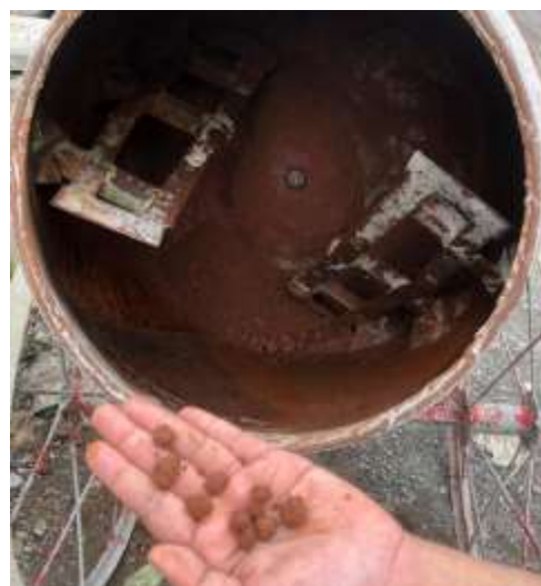
Fig. 5. Pelletization process using mixer rotation
