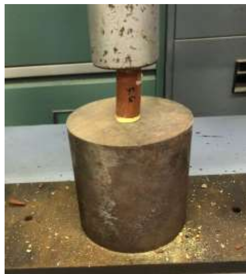
Fig. 7. Single-particle crushing test of ALWA using a Universal Testing Machine
