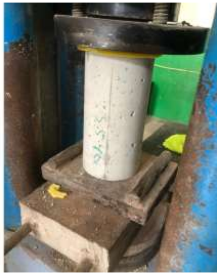
Fig. 8. Concrete compressive strength testing setup
