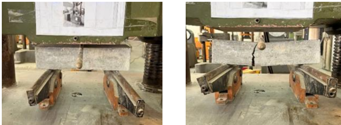
Fig. 7. Flexural strength test set up
