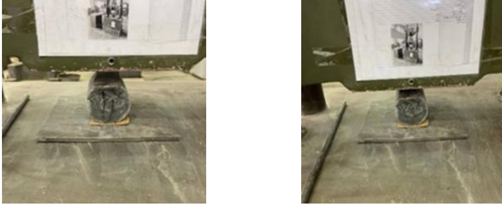
Fig. 8. Splitting tensile strength test set up
