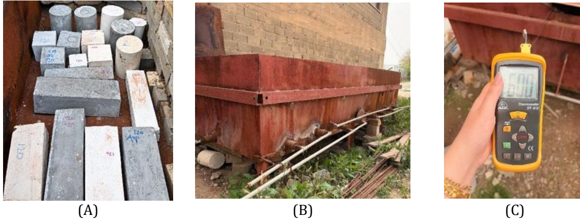
Fig. 11. (A) Placing of specimens in the furnace, (B) Steel furnace, (C) Digital thermometer
