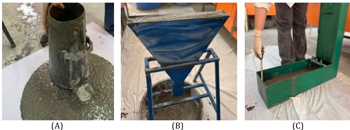
Fig. 5. Fresh properties tests of SCC (A) Slump flow test, (B) V-Funnel test, (C) L-Box test
