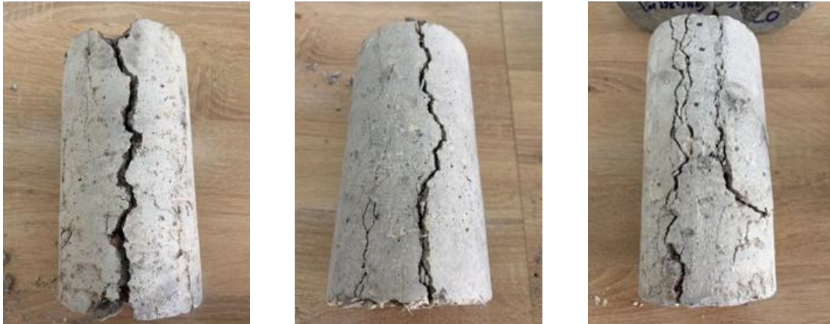
Fig. 20. Cylinders pattern of failure after fire exposure
