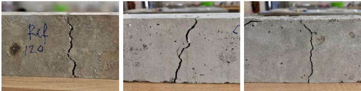
Fig. 17. Prisms pattern of failure after fire test
