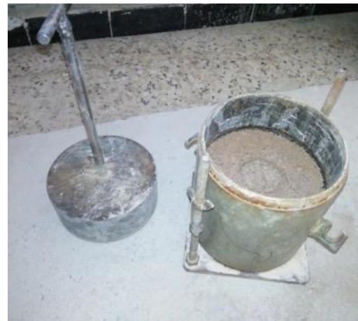
Fig. 7. Sample tested after penetration with the CBR apparatus
