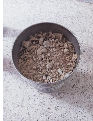
Fig. 5. Granulometric analysis by sieving of EM
