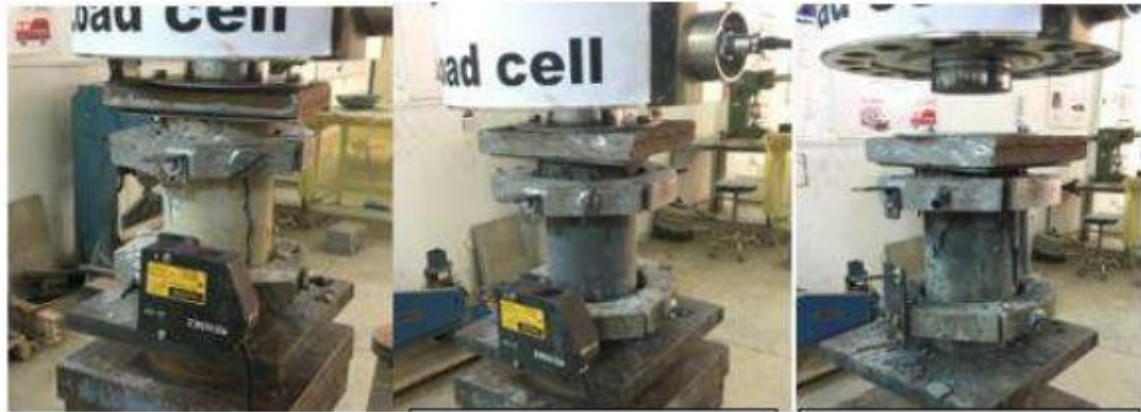
Fig. 12. Progressive compressive failure observed during cylinder testing
