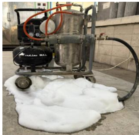
Fig. 1. Foam generator and produced foam
