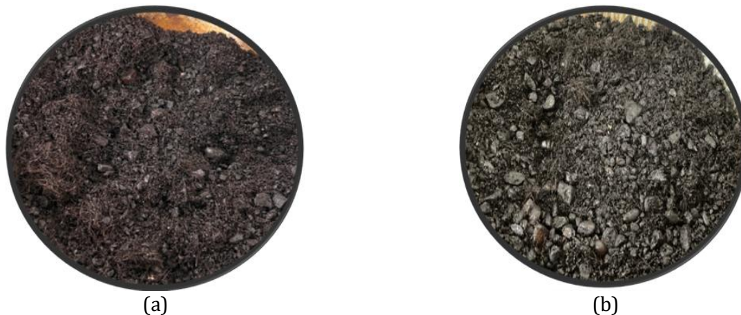
Fig. 6. Visual comparison of sisal-fiber agglomeration at: (a) 0.5% fiber content and (b) 0.7% fiber content, showing more pronounced fiber balling at the higher content
