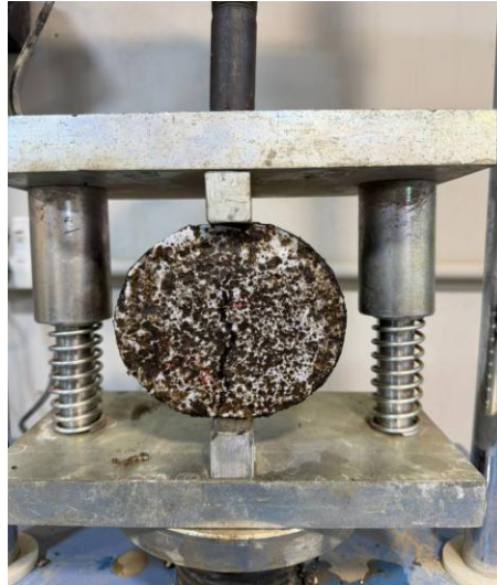
Fig. 5. Experimental setup of the ITS test on a fiber-reinforced WMA specimen
