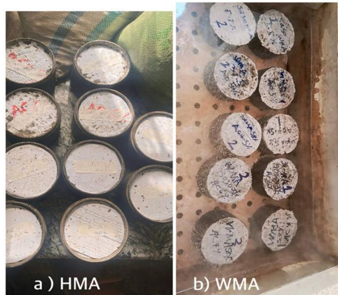
Fig. 3. Laboratory-prepared marshall specimens: (a) Conventional HMA, (b) Warm mix asphalt (WMA-sasobit)
