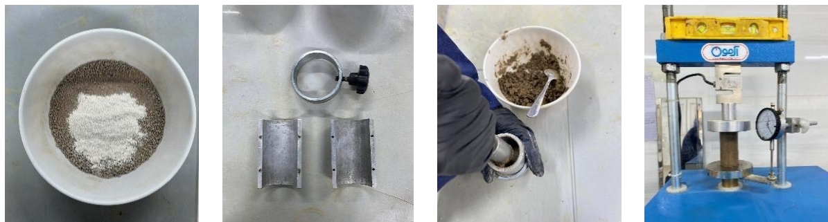
Fig. 4. UCS samples preparing and testing process
