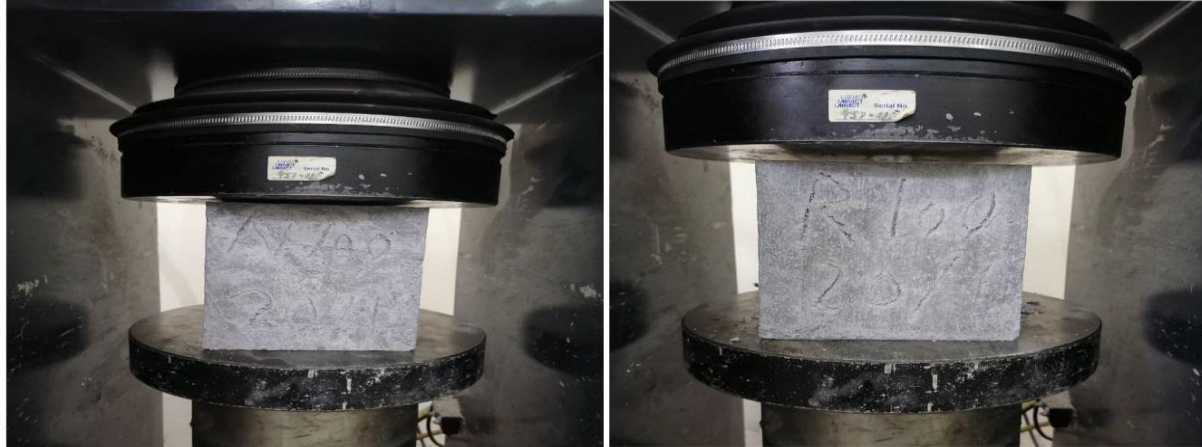
Fig. 4. Cube compression test of hardened concrete
