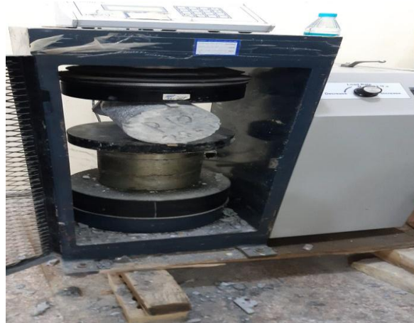
Fig. 6. Splitting tensile strength test of hardened concrete
