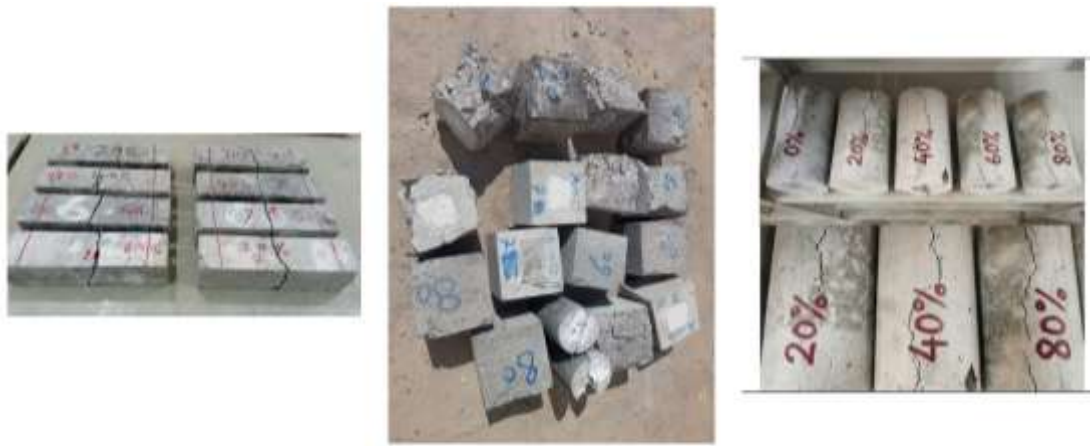
(a) Flexural failure of prisms (b) Representative fractured cubes (c) Splitting-tensile cracking, RCA 0-80%
