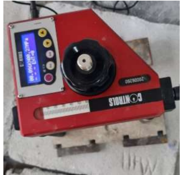
Figure 3. Pull-off strength test
